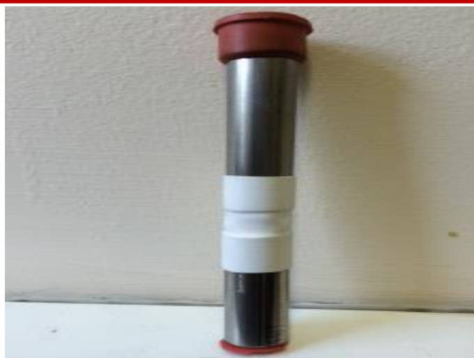
Figure 3. A metal tube for the accumulation and collection of ethylene gas
